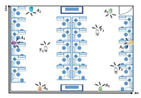
**Figure 5.** Environment 2: Computer laboratory that is equipped with 6 BLE estimates used to estimate 3 tag locations.
