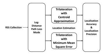
Figure 3. Trilateration Based Localization Model.
