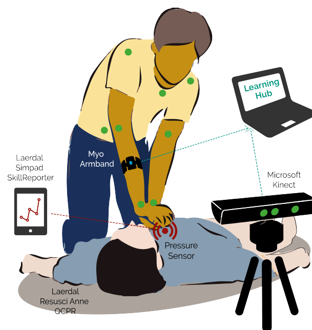
Figure 1. The graphic representation of the experimental setting.
