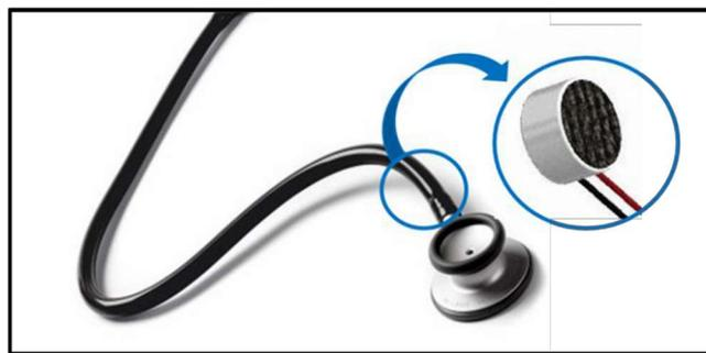
Figure 3. Customized acoustic sensor.
