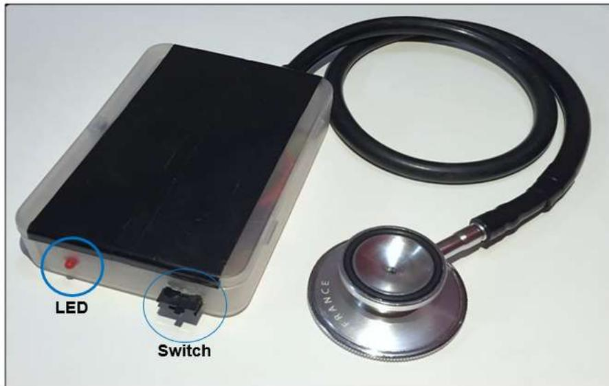
**Figure 5.** Overall implemented phonocardiogram (PCG) signal acquisition system.
