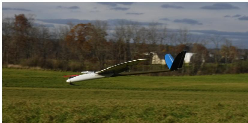
**Figure 9.** The Vulture, a small fixed-wing UAS based on a 2.5 m span model sailplane. It is equipped with an autopilot, onboard computer, and dual power systems permitting 30 min of flight time and more than 10 h of avionics run time. This allows multiple consecutive flights without disrupting the modeling system.
