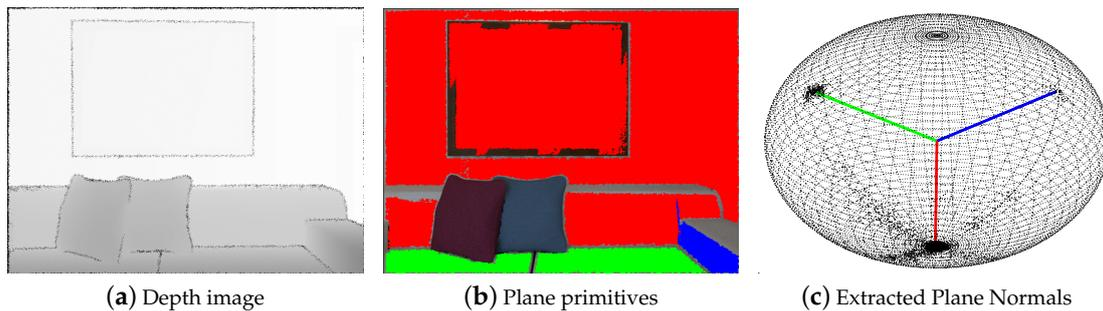
**Figure 4.** Result of the plane normal extraction: (a) depth image of Frame 0 in the 'Living Room 1' sequence of the ICL-NUIM dataset; (b) detected planes using fast plane extraction method; (c) extracted plane normals on the unit sphere. The plane primitives in the image domain and their corresponding extracted normal vectors are in the same color.
