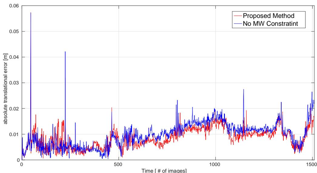
**Figure 7.** Performance evaluation for the MW constraint on the ‘Living Room 0’ sequence. Absolute translational errors for our proposed method with and without the MW constraint are compared.
