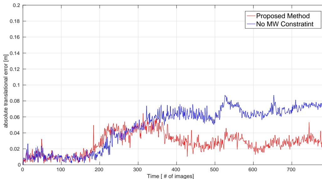
**Figure 9.** Performance evaluation for the MW constraint on the ‘fr3\_struc\_notex\_far’ sequence. Absolute translational errors for our proposed method with and without the MW constraint are compared.
