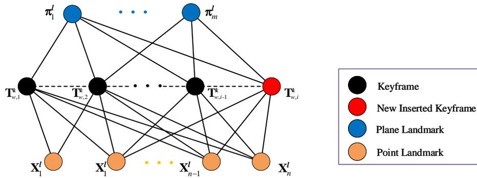
**Figure 2.** Point–plane-based factor graph that is used to represent the local map. Four colors denote four different elements. When a new keyframe (red circle) is inserted, the pose of the keyframes (black circles), point landmarks (blue circles), and plane landmarks (yellow circles) are optimized by minimizing the error cost function constructed by the factor graph.
