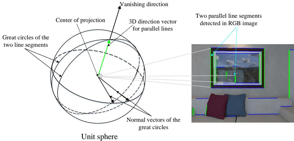
**Figure 5.** Three-dimensional geometric relationship between parallel lines and their vanishing direction. The unit sphere is in the center of a camera projection. Two parallel lines are projected onto the unit sphere as two great circles, and the vanishing direction is obtained by the cross-projection of these two great circles' normal vectors. Two parallel lines and their corresponding vanishing direction are drawn in red.
