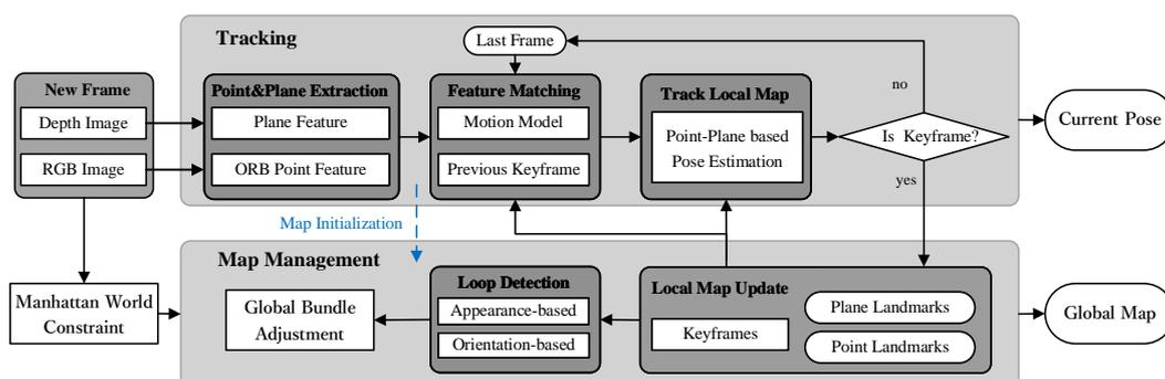
**Figure 1.** Overview of our point–plane-based RGB-D SLAM system. The inputs of the system are the RGB and depth images, and it can output the camera pose and scene’s map. We estimate the camera poses by using the tracked point and plane features. We exploit the point and plane constraints to update the local and global maps. The MW constraint is added to the map management part if the global MW axes are extracted from the first captured RGB-D frame.
