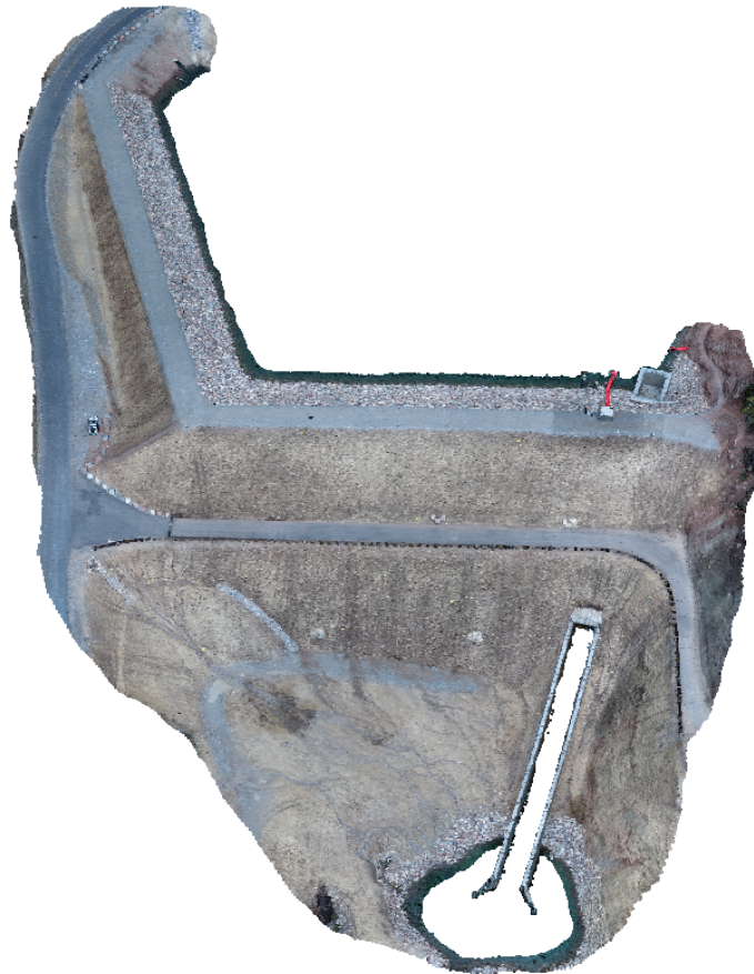
Figure 9. Final model of Tibble Fork Dam built using Agisoft PhotoScan software.
