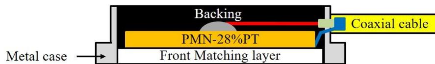
**Figure 5.** Structure of the PMN-28%PT ultrasonic transducer developed for non-destructive evaluation (NDE) of PWR fuel rods.
