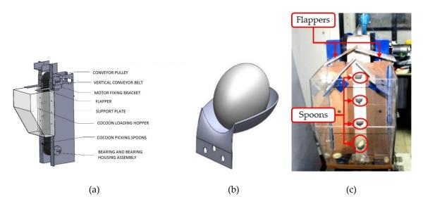
**Figure 7.** (**a**) 3D model of vertical conveyor module (VCM) module; (**b**) 3D model of spoon carrying a cocoon; (**c**) prototype of VCM module.
