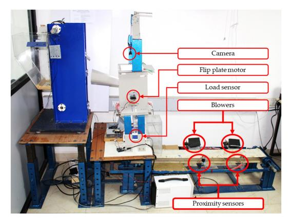
Figure 6. Developed prototype of silkworm cocoons multi-sensor classification system.
