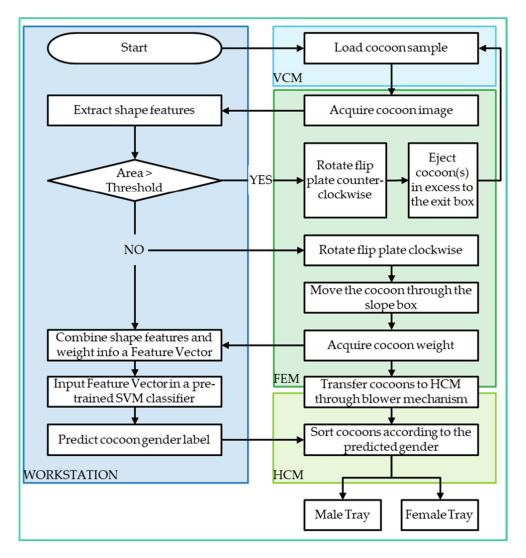
Figure 12. Flow diagram of silkworm cocoons gender classification machine.
