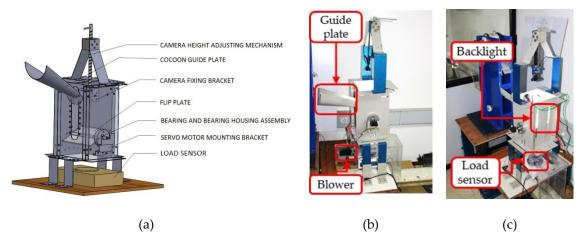
Figure 8. (a) 3D model of FEM; (b,c) prototype of FEM shown in two different angles.
