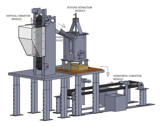
Figure 5. 3D model of silkworm cocoons separating machine.
