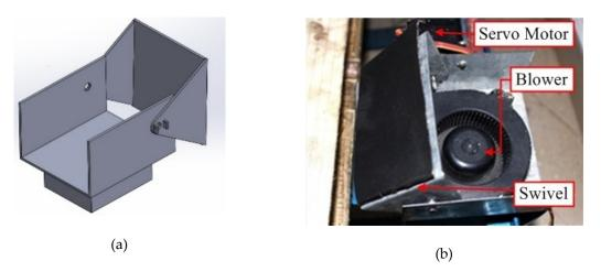
Figure 10. (a) 3D model of air blower frames; (b) developed air blower mechanism.
