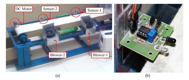
Figure 11. (a) Horizontal Conveyor Module; (b) IR proximity sensor close-up.
