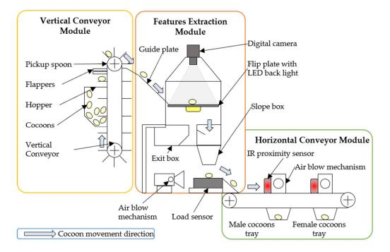
Figure 4. Schematic of silkworm cocoons separating machine.
