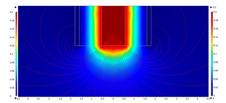
**Figure 4.** The electric field pattern of the fringing field surrounding open-ended coaxial electrodes with 3.6 mmφ for the outer conductor. The color indicates the spatial distribution of potential between zero and 200 mV.
