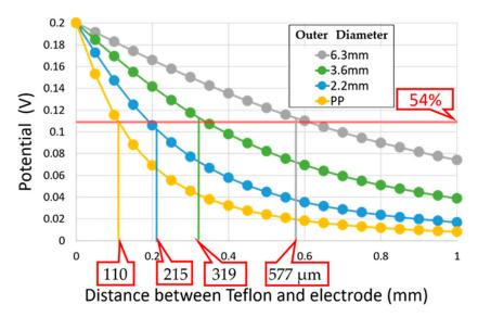
**Figure 5.** Penetration depth determined from potential obtained by the finite element method (FEM) for each electrode.
