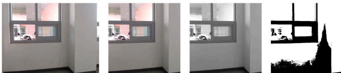
**Figure 9.** Convert process of original image. (a) Original image; (b) crop image; (c) gray-scale image; (d) binary image.
