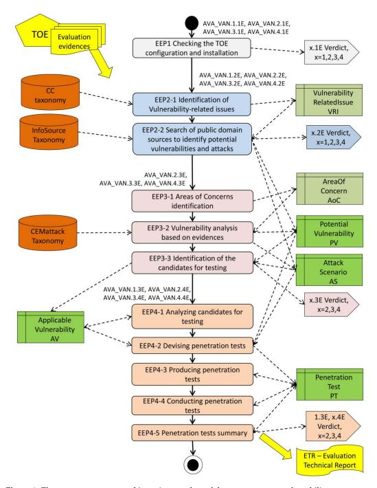
**Figure 1.** Elementary processes and input/output data of the sensor system vulnerability assessment method (SVAM).
