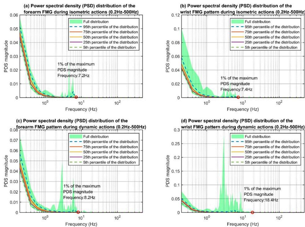
**Figure A1.** Maximum FMG power spectral density (PSD) distributions using Yule–Walker autoregressive method with order of 1000.
