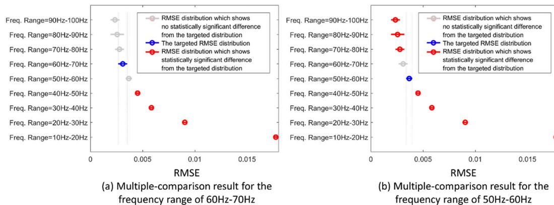
**Figure 7.** RMSE distributions for different resampling frequency ranges. The circle indicates the mean RMSE and the horizontal line shows the  $\pm$  one standard deviations.
