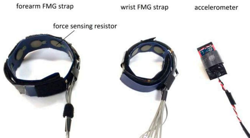
**Figure 2.** FMG and motion sensing devices.
