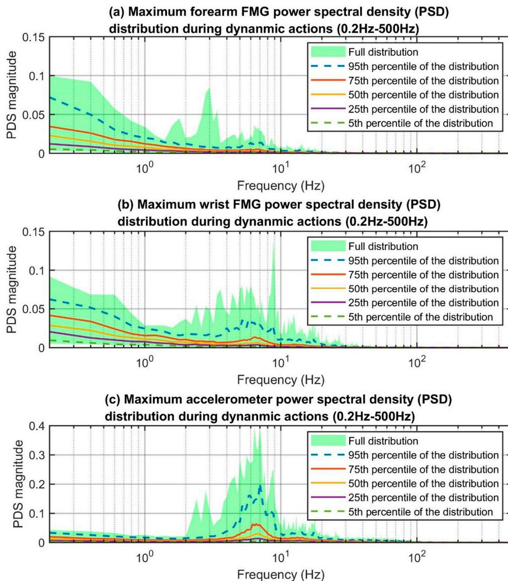
**Figure 9.** Maximum FMG power spectral density (PSD) distribution of FMG and the accelerometer signal during dynamic actions.
