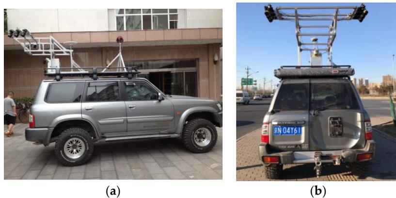
**Figure 1.** Modified mobile-mapping system. (a) Side view. (b) Back view.
