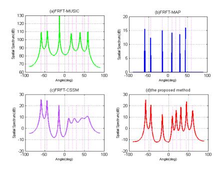
Figure 7. DOFs performance comparison with respect to spatial spectrum when 8 wideband LFM signals impose on the array. (a) FRFT-MUSIC; (b) FRFT-MAP; (c) FRFT-CSSM; (d) The proposed method.
