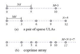
**Figure 1.** The structure of coprime array with M = 3 and N = 5.
