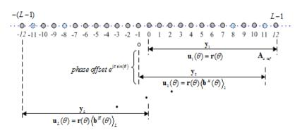
**Figure 4.** The division of sub-array in virtual ULA  $S_U$  with M = 3 and N = 5.
