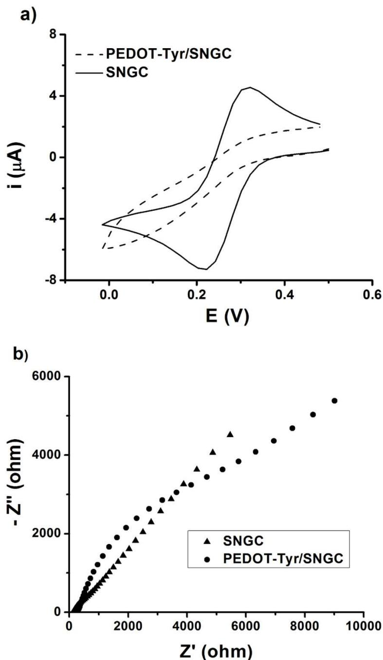
**Figure 1.** Electrochemical characterization of poly(3,4-ethylenedioxythiophene)-Tyrosinase/Sonogel-Carbon (PEDOT-Tyr/SNGC) and Sonogel-Carbon (SNGC) electrodes in an aqueous solution containing 5 mM  $\text{K}_3\text{Fe}(\text{CN})_6$ , and 1 M KCl. (a) Cyclic voltammetry, (b) electrochemical impedance spectroscopy (EIS) spectra recorded in an aqueous solution containing 5 mM  $\text{K}_3\text{Fe}(\text{CN})_6/\text{K}_4\text{Fe}(\text{CN})_6$ , and 1 M KCl.
