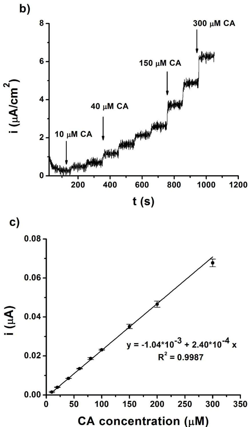
**Figure 2.** (a) Cyclic voltammograms recorded at SNGC and PEDOT-Tyr-SNGC electrodes in a 0.1 M phosphate buffer aqueous solution containing 300  $\mu\text{M}$  caffeic acid, at 50 mV/s potential scan rate; (b) Chronoamperogram corresponding to caffeic acid additions (10, 20, 40, 60, 80, 100, 150, 200, and 300  $\mu\text{M}$ ) at the PEDOT-Tyr/SNGC biosensor; (c) calibration plot with error bars expressed as standard deviation.
