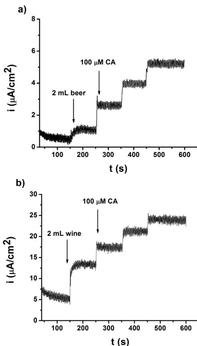
**Figure 3.** (a) Chronoamperogram recorded with the PEDOT-Tyr/SNGC biosensor for beer analysis using the standard addition method (100, 200, and 300  $\mu\text{M}$  CA additions). (b) Chronoamperogram recorded at the PEDOT-Tyr/SNGC biosensor for red wine analysis using the standard addition method for various CA additions (100, 200, and 300  $\mu\text{M}$ ).
