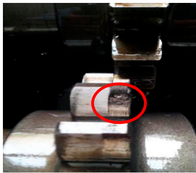
(a) Spalling failure of gear
