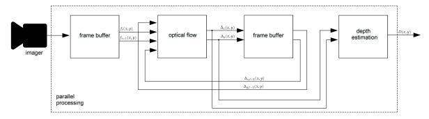
Figure 1. Block diagram of the proposed algorithm.
