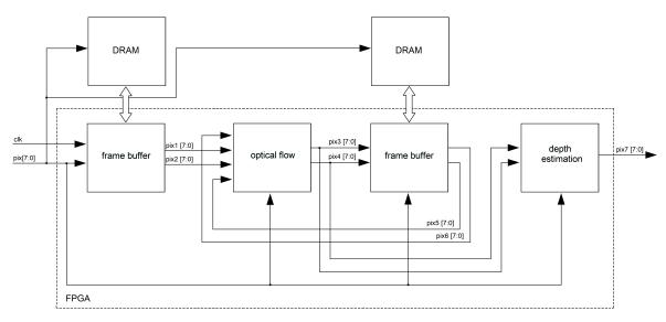
Figure 8. FPGA architecture for the proposed algorithm.
