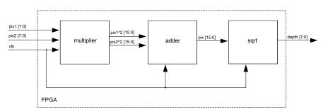
Figure 13. FPGA architecture for the "depth estimation" unit.
