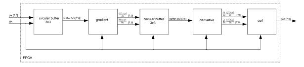
Figure 12. FPGA architecture for the "curl" unit.
