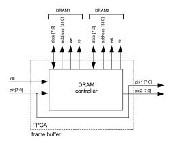
**Figure 9.** FPGA architecture for the "frame buffer" unit. Two external memories configured in switching mode makes it possible to store the current frame (time *t*) into a DRAM configured in write mode, while another DRAM (in read mode) deliver pixel flow for a previous frame (frame at time t - 1).
