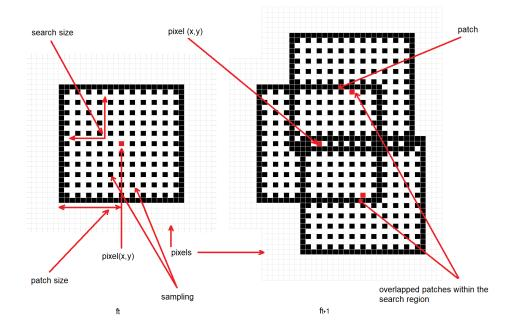
**Figure 5.** The proposed optical flow algorithm formulation: patch size = 10, search size = 10, and sampling value = 2. For each pixel in the reference image  $f_t$ , n overlapped regions are constructed in  $f_{t+1}$ , and the n region center that minimizes or maximizes any similarity metric is the tracked position (flow) of the pixel (x, y) at  $f_{t+1}$ .
