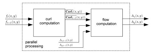
**Figure 2.** The optical flow step: first, curl images  $(\overline{\mathbf{Curl}_t}(x, y))$ ,  $(\overline{\mathbf{Curl}_{t+1}}(x, y))$  are computed. Then, given the curl images for two consecutive frames, pixels displacements  $\Delta_x(x, y)$ ,  $\Delta_y(x, y)$  (optical flow for all pixels in the reference image) are computed using a dynamic template based on the optical flow previously computed  $(\Delta_{x,t-1}(x, y), \Delta_{y,t-1}(x, y))$ .
