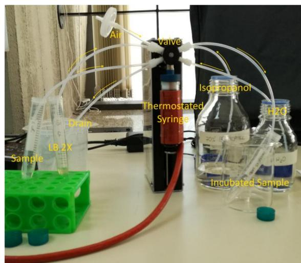
Figure 14. Configuration of the thermostated syringe.
