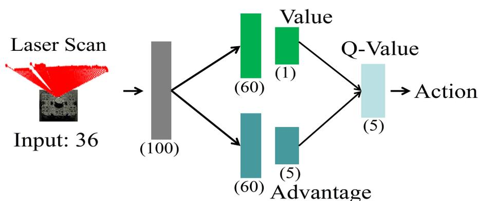
**Figure 2.** Deep double Q network (D3QN) network structure. Input is a 36-dimensional vector representing the laser range findings sampled from the raw laser scan between  $-180^\circ$  and  $180^\circ$  at 5 degree resolution. The output is a 5-dimensional vector representing the Q-values of the state-action pairs.
