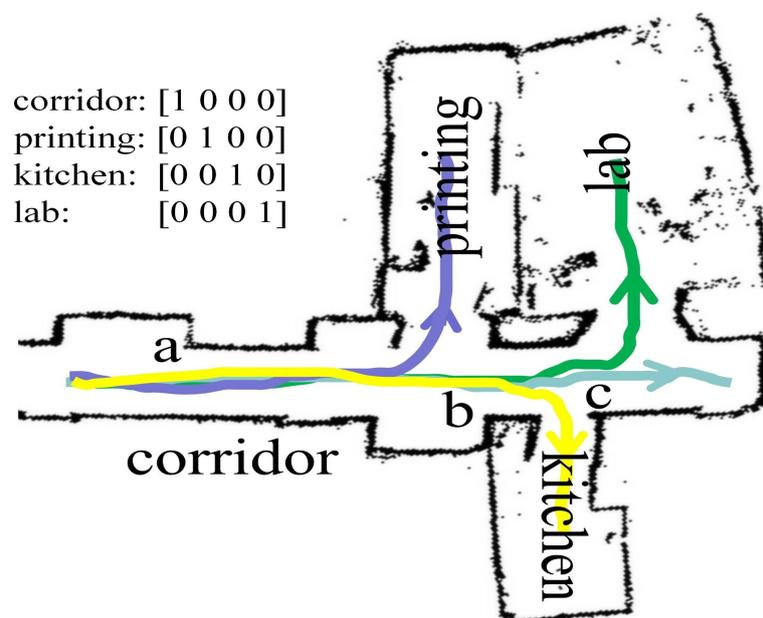
**Figure 5.** The moving trajectories predicted by the goal-directed end-to-end network towards different goals in the real world. The light blue line represents the trajectory to the corridor end. The yellow line represents the trajectory to the kitchen. The purple line represents the trajectory to the printing room. The green line represents the trajectory to the student lab.
