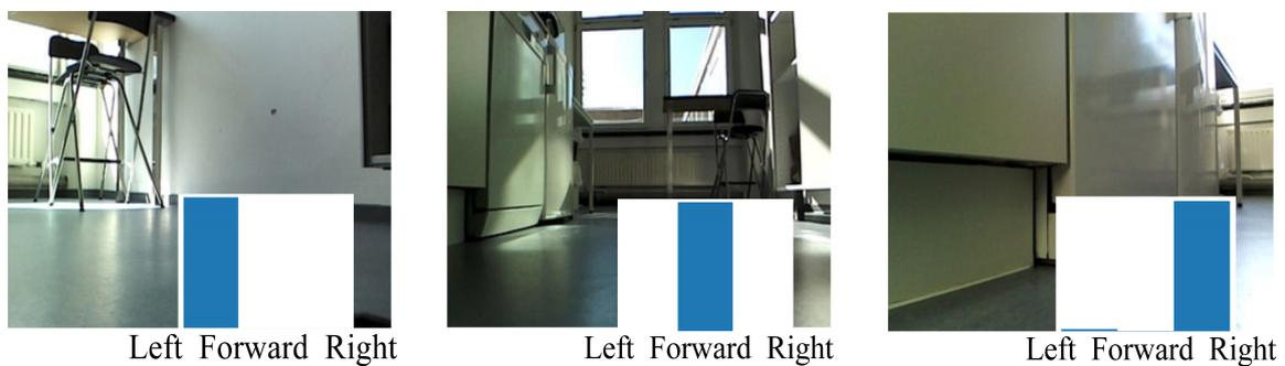
**Figure 4.** An example of the output of the end-to-end network. The underlying bars demonstrate the action probability predicted by the network.
