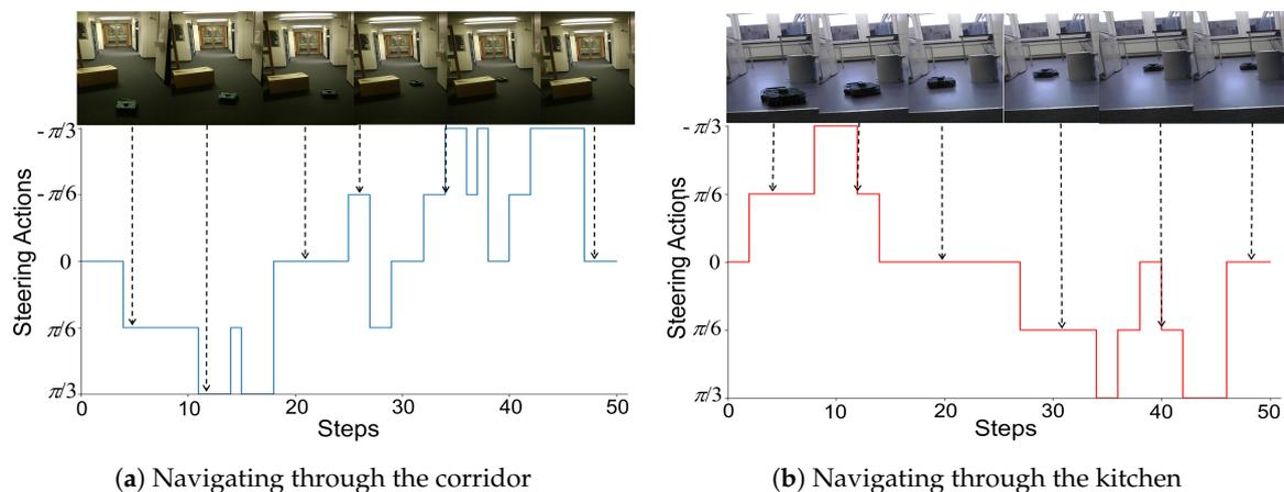
**Figure 10.** Action choices of the local planner during local navigations. The curve below the image streams shows the steering action selected by the local planner at each step.
