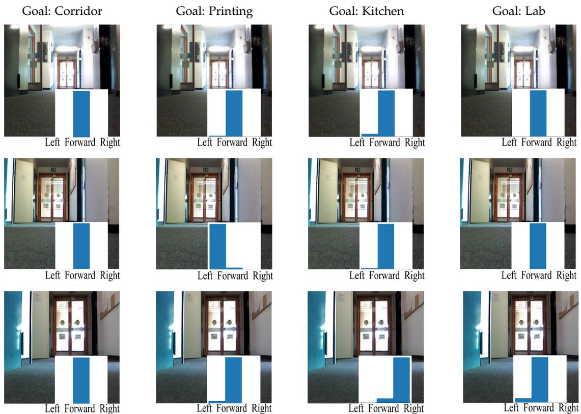
**Figure 6.** The goal-directed end-to-end network results for three representative positions in the environment. The underlying bars demonstrate the action probability predicted by the network. The rows represent the camera image at three positions sampled from the area a, b, c in Figure 5. The 4 columns represent the 4 different goals: The corridor, the printing room, the kitchen, and the lab.
