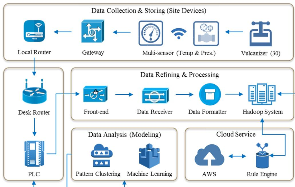
**Figure 2.** Sensor-based infrastructure.
