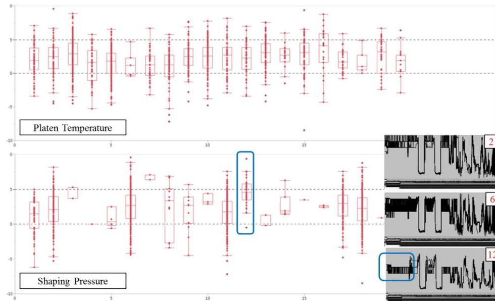
**Figure 6.** Box plot from the clusters of platen temperature and shaping pressure.
