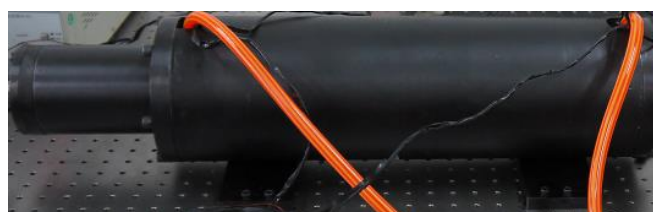
Figure 10. Experimental prototype of a giant magnetostrictive actuator.
