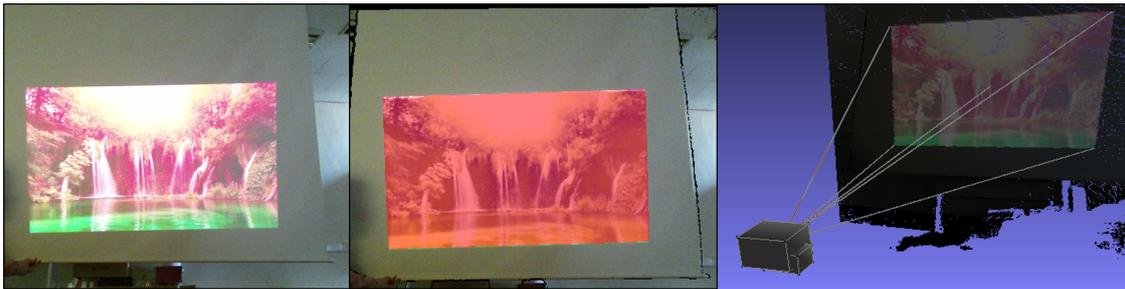
**Figure 5.** An example of the projection surface masks  $\mathbb{M}_s(x, y)$  obtained by Equation (4). The left image is a captured image with the projection and its background. The red region of the center image represents the projection surface masks. The right image shows the projection surface masks (colored regions) in 3D projector coordinates with five projection rays (white lines) at the boundaries and center.
