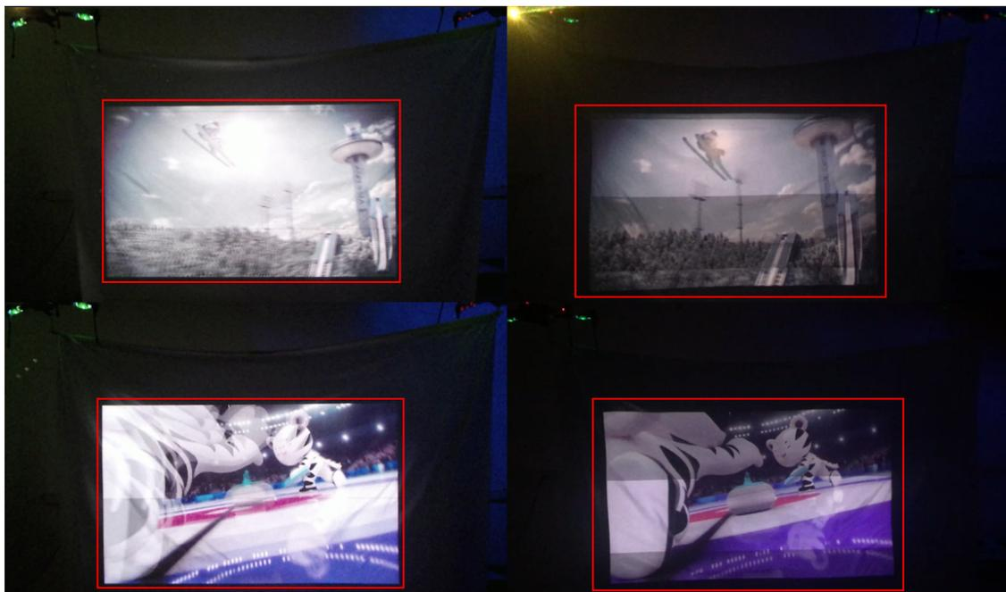
**Figure 11.** DIW results from dynamic non-planar surfaces generated from UAVs and a lightweight canvas. The left column depicts the result obtained with the proposed method and the right column shows the output of a conventional projector.
