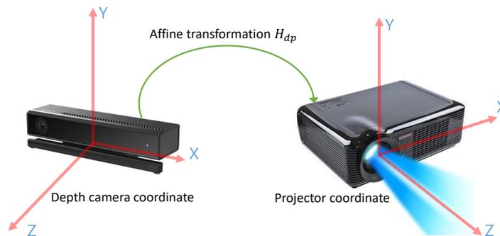
**Figure 2.** An example of the relation between the depth camera and projector coordinates, where the affine transform matrix  $\mathbf{M}_{dp}$  transforms the depth camera coordinates ( $\mathbf{P}_d$ ) into the projector coordinates ( $\mathbf{P}_p$ ).
