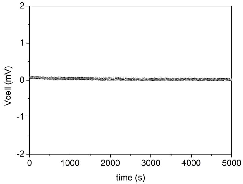
Figure S5 Sensor baseline when exposed to 6% of O<sub>2</sub> balanced with argon at 550 °C. The sensor consists of Fe<sub>0.7</sub>Cr<sub>1.3</sub>O<sub>3</sub>/8YSZ as WE and Pt as RE
