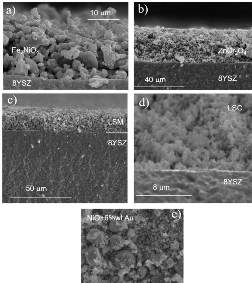
Figure S2 SEM image of the device cross-section showing the interface WE-electrolyte corresponding to a)  $\text{FeNiO}_4$ , b)  $\text{ZnCr}_2\text{O}_4$ , c) LSM and d) LSC. On the other hand, e) shows the NiO+5%wt Au surface.
