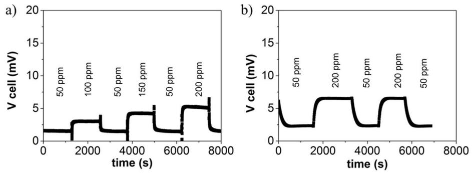
Figure S4 Response transient to C<sub>2</sub>H<sub>4</sub> of the sensor employing as WE: a) LSC and b) LSC/8YSZ (1:1 vol.)
