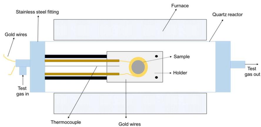
Figure S1 Experimental set-up used to measure sensor response
