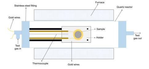
Figure S1 Experimental set-up used to measure sensor response
