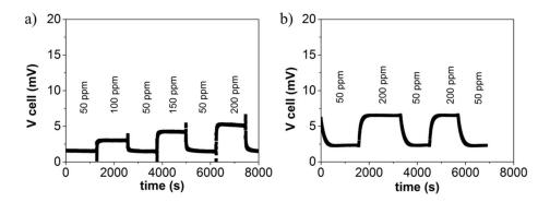
Figure S4 Response transient to  $C_2H_4$  of the sensor employing as WE: a) LSC and b) LSC/8YSZ (1:1 vol.)
