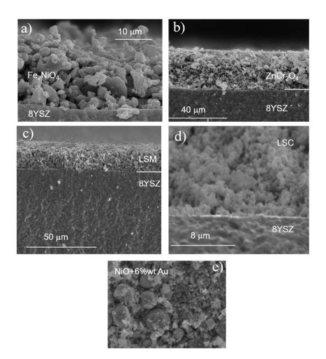
Figure S2 SEM image of the device cross-section showing the interface WE-electrolyte corresponding to a) FeNiO<sub>4</sub>, b)  $ZnCr_2O_4$ , c) LSM and d) LSC. On the other hand, e) shows the NiO+5% wt Au surface.
