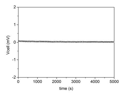
Figure S5 Sensor baseline when exposed to 6% of O<sub>2</sub> balanced with argon at 550 °C. The sensor consists of Fe<sub>0.7</sub>Cr<sub>1.3</sub>O<sub>3</sub>/8YSZ as WE and Pt as RE
