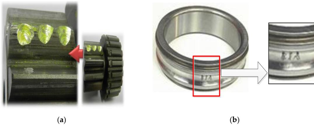
Figure 4. The fault modes: (a) sun gear chipped; (b) planetary gear bearing with inner-race fault.
