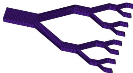
Figure 8. Finite element model of the tube.
