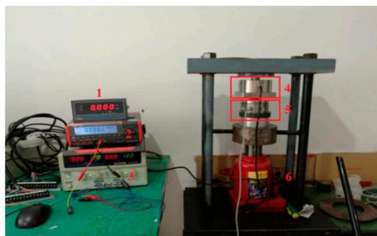
**Figure 15.** Experimental setup. (1) Displayer 1; (2) Displayer 2; (3) DC power; (4) Acoustic filtering sensor; (5) Standard sensor; (6) Hydro-cylinder.
