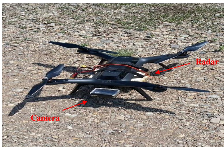
Figure 10. Attachment of the camera and radar to the SOLO quadcopter.
