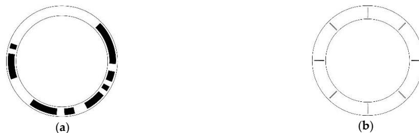
**Figure 7.** Disc pattern and slit disc of the prototype using a length-8 period-128 STGC: (a) Schematic of the coding disc, where the white area indicates “0”, and the black area indicates “1”; (b) Schematic of the slit disc, where the eight slits are arranged right over the eight reading heads. This disc except the eight slits should be black, but to show the slits clearly we use white instead.
