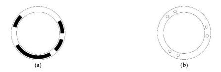
**Figure 5.** Disc pattern and reading head distribution of absolute encoder using a length-6 period-48 twin-necklace ordering STGC: (**a**) Schematic of the coding disc, where white area indicates "0", and the black area indicates "1"; (**b**) Schematic of the reading disc, where the six small circles denote the six reading heads, and the sub-cycle of the head interval is two.
