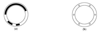
**Figure 3.** Disc pattern and reading head distribution of absolute encoder using a length-6 period-36 necklace ordering STGC. (**a**) Schematic of the coding disc, where white the area indicates "0", and the black area indicates "1"; (**b**) Schematic of the reading disc, where the six small circles denote the six reading heads and are evenly distributed around the whole coding track.
