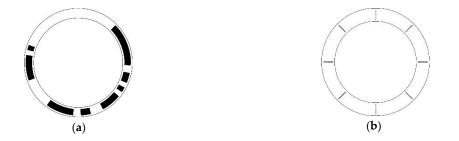
**Figure 7.** Disc pattern and slit disc of the prototype using a length-8 period-128 STGC: (**a**) Schematic of the coding disc, where the white area indicates "0", and the black area indicates "1; (**b**) Schematic of the slit disc, where the eight slits are arranged right over the eight reading heads. This disc except the eight slits should be black, but to show the slits clearly we use white instead.
