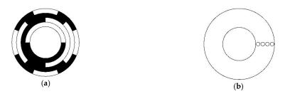
**Figure 1.** Disc pattern and reading head distribution of absolute encoder using a length-4 Gray code: (a) Schematic of the coding disc, where the white area indicates "0", and the black area indicates "1"; (b) Schematic of the reading disc, where the four small circles denote the four reading heads corresponding to the four coding tracks.
