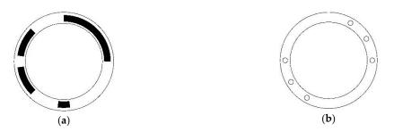
**Figure 6.** Disc pattern and reading head distribution of absolute encoder using a length-6 period-48 triplet-necklace ordering STGC: (**a**) Schematic of the coding disc, where the white area indicates "0", and the black area indicates "1"; (**b**) Schematic of the reading disc, where the six small circles denote the six reading heads, and the sub-cycle of the head interval is three.
