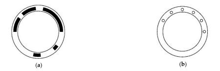
**Figure 4.** Disc pattern and reading head distribution of absolute encoder using a length-6 period-36 necklace ordering STGC. (a) Schematic of the coding disc, where the white area indicates "0", and the black area indicates "1; (b) Schematic of the reading disc, where the six small circles denote the six reading heads and are evenly distributed around the half coding track.
