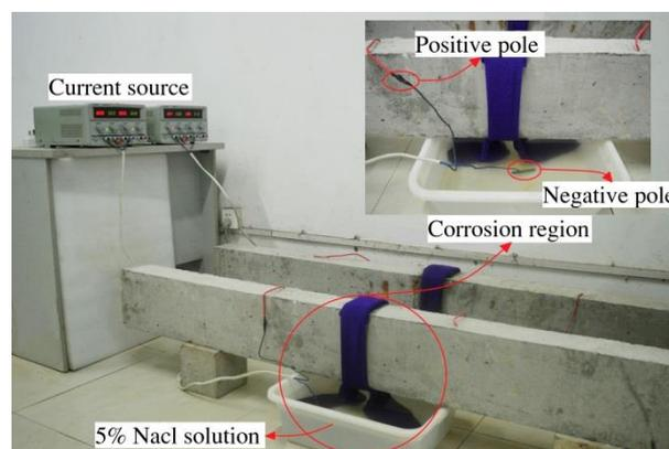
Figure 2. Layout of the corrosion device.
