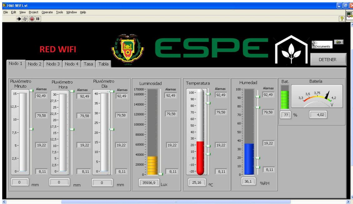
**Figure 5.** Monitoring of greenhouse variables, battery condition, alarms, data rate, and table for the WiFi network.
