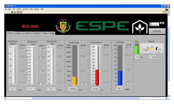
**Figure 5.** Monitoring of greenhouse variables, battery condition, alarms, data rate, and table for the WiFi network.
