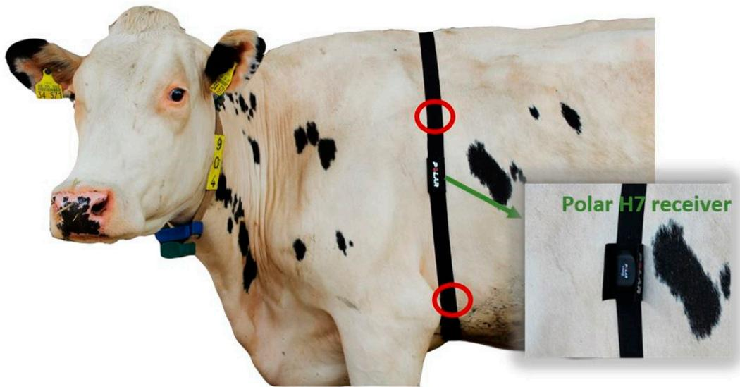
**Figure 1.** Dairy Cow I equipped with the Polar equestrian chest belt and Polar H7 receiver; red circles mark the placement of the electrodes.
