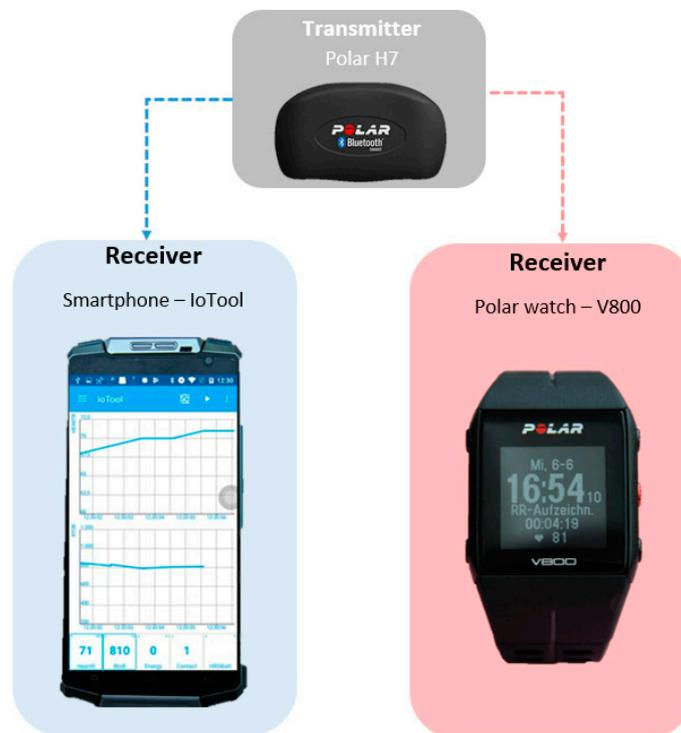
**Figure 2.** Schematic diagram of the experimental setup with Polar H7 transmitter, receiver smartphone IoTool application (left) and receiver Polar watch V800 (right).
