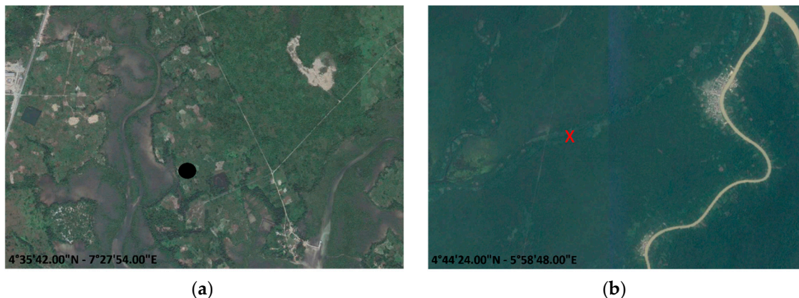
Figure 13. Two examples of false positives by: (a) RST-FLARE; (b) VNF. In background are GoogleEarth® images of (a) 19/12/2013 and (b) 23/12/2015. The visual inspection has been carried out for the whole temporal period exploiting the GoogleEarth timeline tool (clock button).
