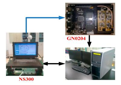
Figure 2. Structure of the highly-dynamical scene experiment scheme.
