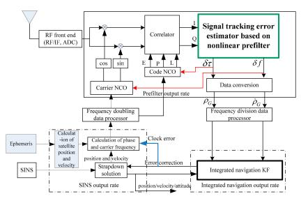
Figure 1. SINS/GPS federated ultra-tightly coupled structure based on double loop.
