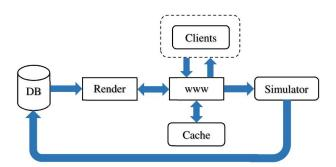
**Figure 9.** Tile map server architecture: tiles are requested from the web page server that either return a cached image or ask the rendering engine to compose it from a data base of geographical objects.
