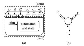
**Figure 12.** Cell node representation: (**a**) is the internal architecture with an automaton (*rule*) operating on incoming values and local stimuli (*stim*), based on a local set of variables, filling output communication buffers. Communications (*com*) are operated to and from the input and output buffers; (**b**) is the external point of view that only shows bidirectional links of a cell node.
