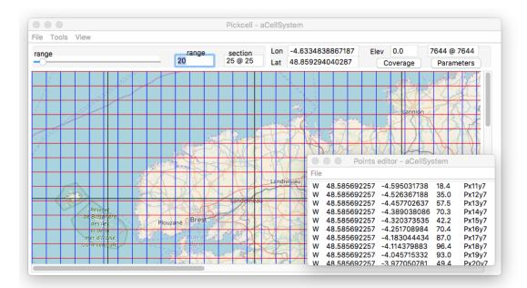
**Figure 10.** Presentation of a cell system organization over the tiles of Figure 8. Each cell has an identity produced from its location inside the window, and a geographical location. The text window bottom right also displays a plus parameter for the elevation. The cell size is  $25 \times 25$  pixels, representing 7644 m.
