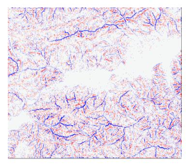
**Figure 2.** TPI terrain complexity for the river Soummam in Algeria (see also Figure 5). Red lines represent higher points, difficult to overcome and blue lines are for lower points, difficult to reach. The white zone signals a flat ground without remarkable obstacles, the case of Soummam banks. This grid is  $262 \times 226$  points, representing  $30 \times 25$  km.
