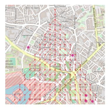
**Figure 16.** Directed BSF is a distributed parallel algorithm able to manipulate data on grid cells. Its aim is to mimic point-to-point radio links adopting the LoS condition. Segmented lines are laid on a map to represent how cells forward incoming signal gradually from a root cell (x = 10, y = 1) to definite directions.
