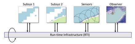
**Figure 1.** Federation of two complementary cellular subsystems, a sensor network, and some display for observation. A software bus (RTI) provides services for data exchanges, sequencing and synchronization. This framework is called *High Level Architecture*, standardized as IEEE Std 1516–2000 [5].
