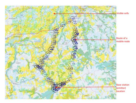
**Figure A7.** The base station (emitter) is located on top of the mountain (latitude: 48.4051306, longitude: -3.9077762, elevation: 345 m). A receiver is placed on a car (receiver) traveling around the area with many hills, valleys, and big trees. From simulation results, places (cells) are able to receive the radio signal highlighted in yellow. Blue circles show points where the receiver successfully obtained messages in our actual measurement.
