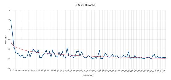
**Figure A8.** Obtained received signal strength indicator (RSSI) values for experiment in our actual measurement at the Roc'h Trevezel. RSSI values decay as a negative exponential function of distance. The complex terrains in this area seriously impact the quality of radio links.
