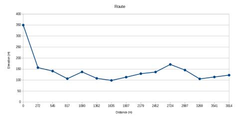
**Figure 15.** A profile obtained along a route. Let's assume that an emitter located on the furthest left of the chart, with a distance of 0 m, an elevation of 350 m. According to LoS condition, three points at distances 2997 m, 3269 m and 3541 m seem unable to receive the signal from the emitter.
