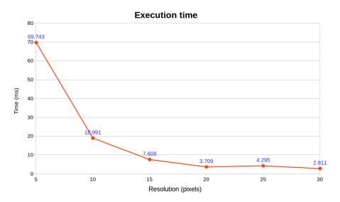
**Figure A9.** Chart of radio coverage execution times for different resolutions of cell from 5 to 30 pixels. This statistics was recorded for the performance on a PC equipped Core i7-7700K CPU@4.20GHz  $\times$  8, 16 GiB DDRAM, card NVidia GeForce GTX 1070 (1920 CUDA cores).
