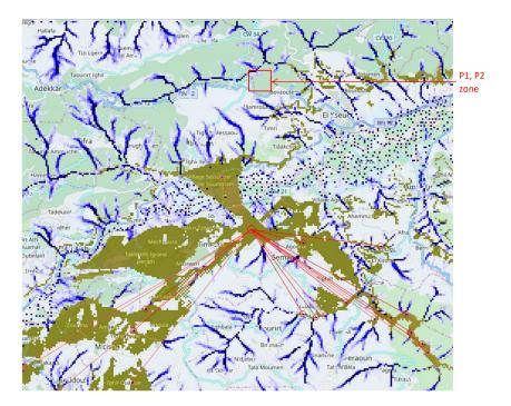
**Figure 7.** Heavy rainfalls context: a physical simulation produced positions with the risk of flash flooding (dark blue color). The communication coverage of a base station with a star network is predicted for sensor nodes monitoring level of water in these positions. An algorithm selects reachable sensor positions from a network sink, sorts, then extracts 15 positions according to the flooding result simulation. More details about accuracy are given in Section 3.
