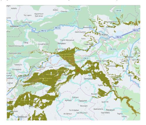
**Figure 5.** Display of a radio coverage for an emitter (red point), located above the Soummam (36.622141028, 4.799995422), elev:165.0 m. Note that geographic positions are proposed in (lat, long) form compatible with familiar map navigators. Coverage is shown in dark yellow, spreading over 30 km on the zone width. This location was chosen at random, giving a percentage of 32% grid points receiving the long-range signal.
