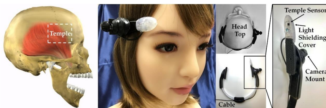
Figure 1. Mouthwitch external appearance and attachment diagram. When performing the operation of opening and closing the mouth, the temporal muscle, which is one of the muscles that moves the chin, is extended and contracted. The mouthwitch, through the right temporal muscle movement, measures the movement of the skin near the right temple using an optical sensor (temple sensor). This temple sensor is equipped with an infrared LED and phototransistor, and the movement of the temporal muscle is measured by infrared light being projected to the skin near the right temple, and this reflected light is received by the phototransistor. This temple sensor is attached to the head-mounted equipment shown in Figure 2, to measure the movement of the skin near the right temple of the test subject. The temple sensor is covered using a light-shielding cover to prevent excess environmental light (direct sunlight, etc.) from entering the phototransistor. The weight of the head-mounted equipment is 82 g. The cable stretching from the head-mounted equipment is connected to a microprocessor for processing the signal results and outputting the shutter operation signal, speakers, and a power supply.
