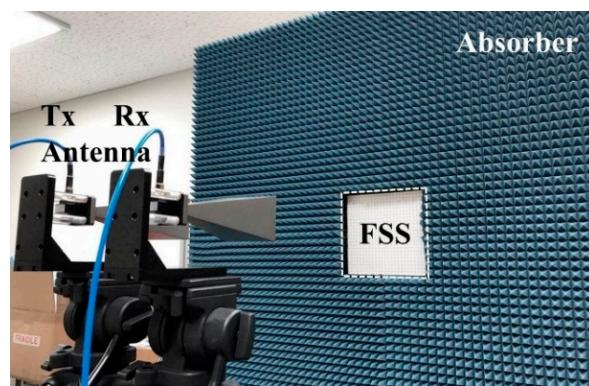
**Figure 5.** Frequency reflection characteristic measurement setup.
