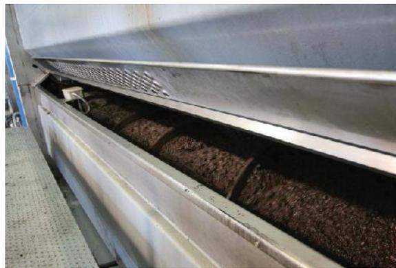
Figure 1. Industrial thermomixer in the virgin olive production process [7].
