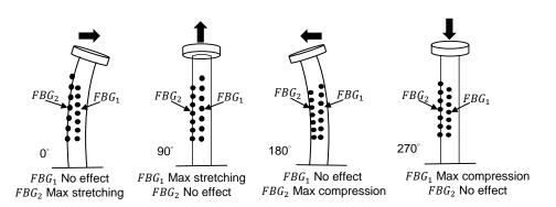
Figure 4. Sensing concept for measuring wind direction.
