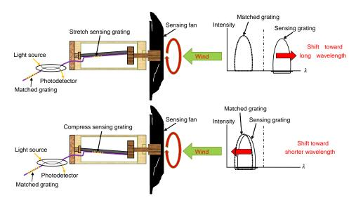
Figure 2. Sensing concept for measuring wind speed.
