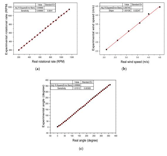
**Figure 9.** Relationship curves between the real and experimental (**a**) rotational speed, (**b**) wind speed, and (**c**) wind-direction angle.
