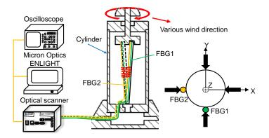
Figure 5. Experimental setup for measuring wind direction.
