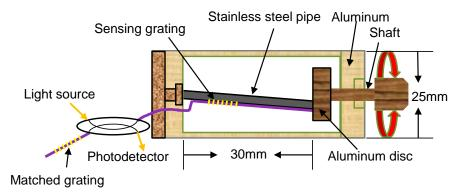
Figure 1. Configuration of the wind-speed sensing head.
