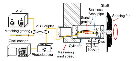
Figure 3. Experimental setup of the sensing head for measuring wind speed.
