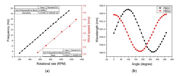
**Figure 8.** Plots of (**a**) frequency and wind speed versus rotational speed and (**b**) grating wavelength shift versus wind-direction angle.
