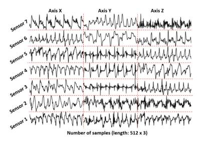
**Figure 2.** Raw acceleration plot of time domain: segment length 512 and sampling rate 50 Hz (the dotted lines are added manually for better clarification; image resolution is  $512 \times 512$  pixels).
