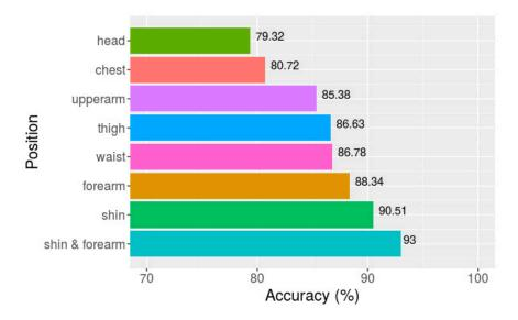
**Figure 7.** Overall classification accuracies of eight activities based on data from seven single positions and two combined positions.
