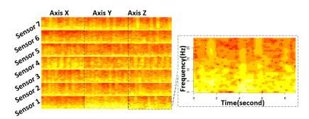
**Figure 4.** Spectrogram plot of the acceleration data. The segment length is 512 and the sampling rate is 50 Hz, with a short-time Fourier transform (STFT) window length of 64 STFT and an overlap length of 60 STFT (image resolution  $336 \times 350$  pixels).
