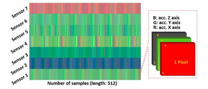
**Figure 3.** Multichannel RGB color plot on time domain. The segment length is 512 and the sampling rate is 50 Hz (image resolution  $512 \times 7$  pixels).
