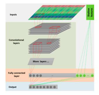
Figure 5. Workflow of deep convolutional neural network (CNN) models.
