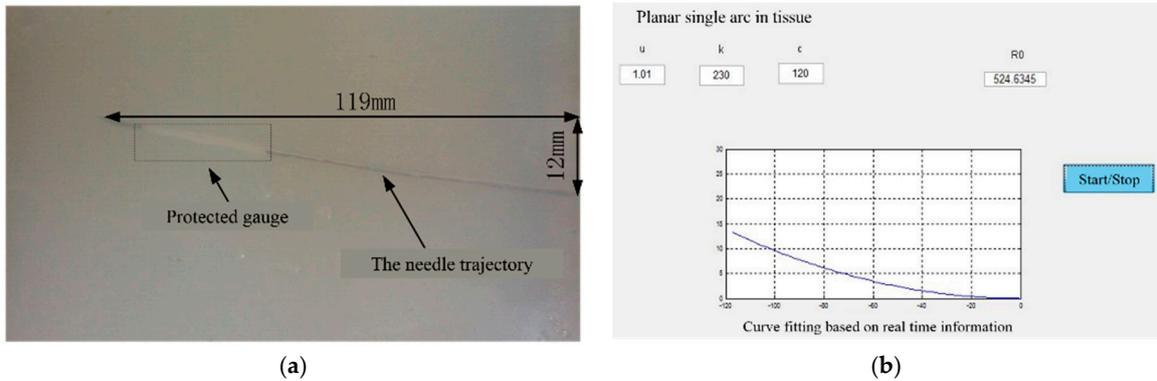
Figure 16. (a) Experiment of needle in tissue; (b) experiment of needle in the computer image.
