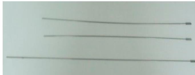
**Figure 2.** Flexible needles with a bevel tip.
