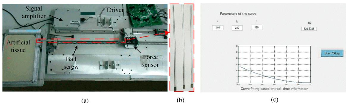
**Figure 1.** The experiment setup. (a) The hardware configuration; (b) The flexible needles used; and (c) The GUI.
