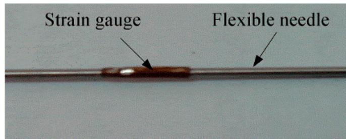
**Figure 4.** Needle with a strain gauge.
