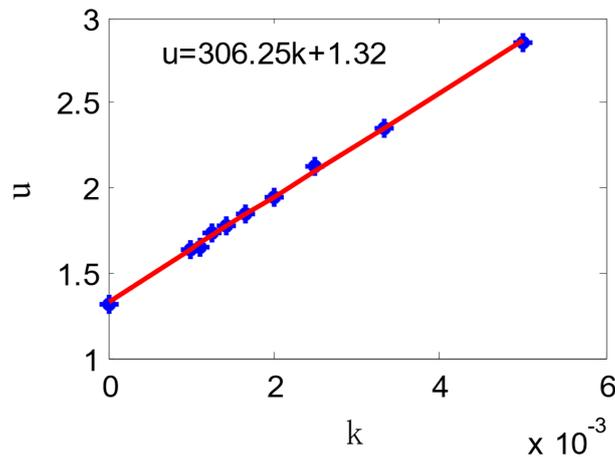
Figure 13. Voltage-curvature relation curve.
