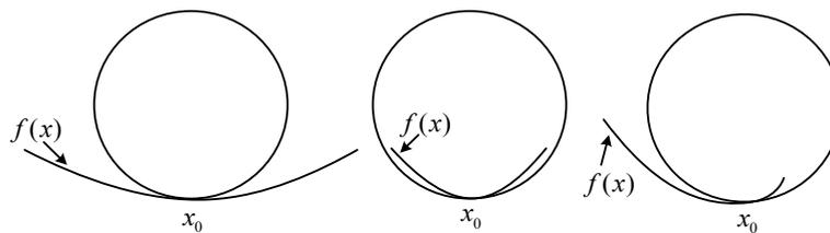
Figure 10. The position relations between a circle of curvature and the curve.
