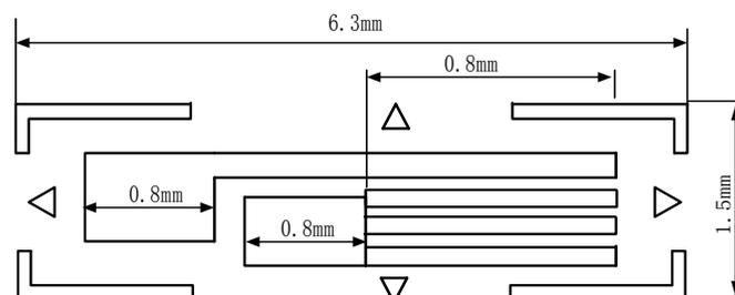
**Figure 3.** The size of the resistance strain gauge.
