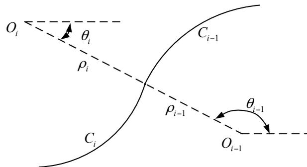
**Figure 8.** The situation when an anticlockwise arc is followed by a clockwise arc.
