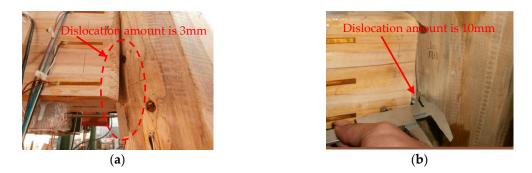
**Figure 16.** Measured dislocation with a: (**a**) loading amplitude of 80 mm; (**b**) loading amplitude of 160 mm.
