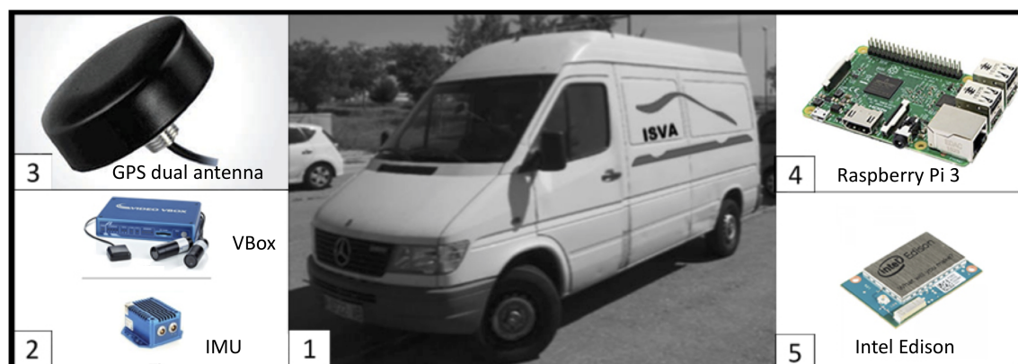
Figure 2. Experimental testbed installed in Mercedes Sprinter van (1) with the ground truth kit (2, 3), Raspberry Pi and Intel Edison kits (4, 5).
