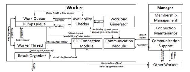
Figure 1. The overall design of HeaLow.
