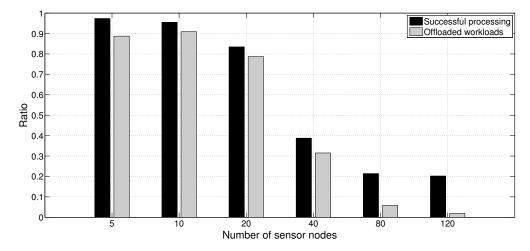
Figure 5. The successfully processed and offloaded amount in a sensor network environment.
