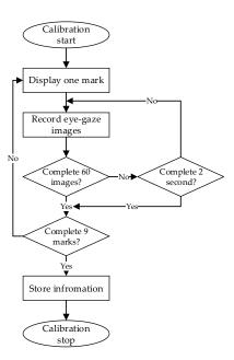
Figure 6. Initial calibration step.
