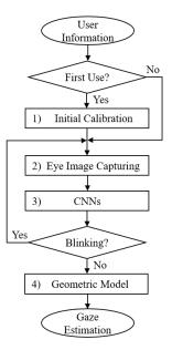
Figure 4. Workflow of the proposed gaze-tracking method.
