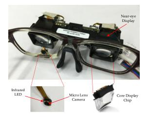
Figure 2. Gaze-tracking device and near-eye viewing device.
