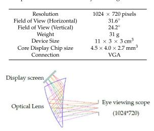
Table 2. The performance of the near-eye viewing device in Etracker.
