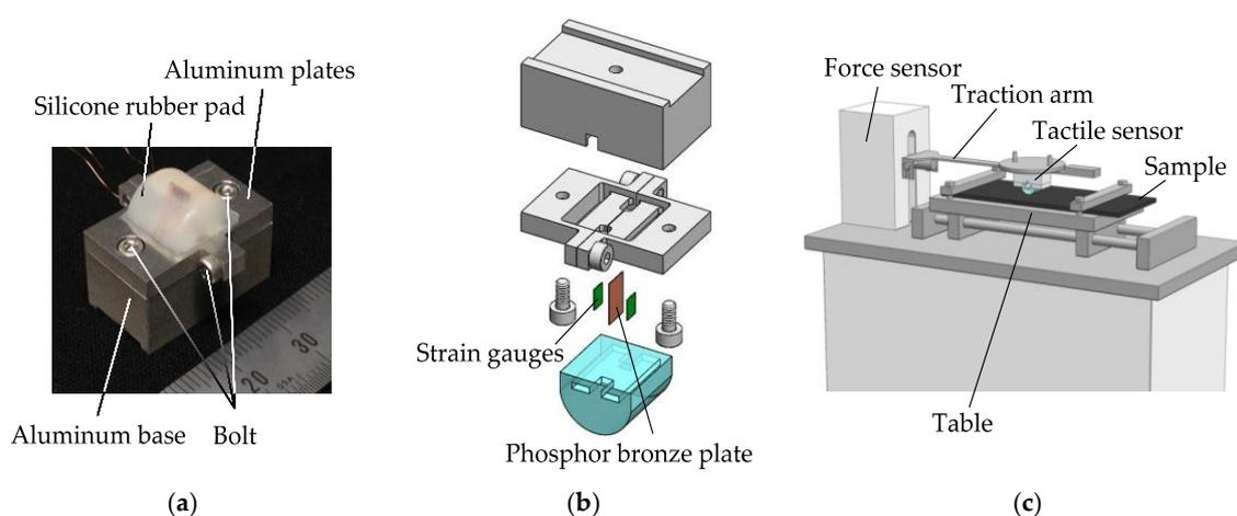
**Figure 2.** Tactile sensing system with developed tactile sensor. (a) Actual image of the sensor; (b) exploded view drawing of the sensor; and (c) overall view of the sensing system. The drawing in (c) shows the tactile sensor runs over a sample as a result of the sliding of the table. The strain gauges of the sensor detect vibration, while the force sensor measures the tangential force.
