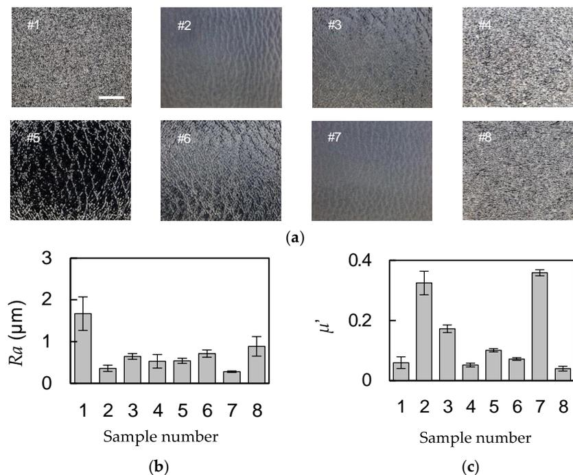
**Figure 1.** The information of plastic test samples. (a) The enlarged views (Scale bar: 5 mm); (b) arithmetic average roughness,  $R_a$  (mean  $\pm$  SD,  $n = 10$ ); and (c) dynamic friction coefficient,  $\mu'$  (mean  $\pm$  SD,  $n = 10$ ). Materials of the plates are: #1; polystyrene, #2; unknown, #3; polypropylene, #4; polyethylene, #5; polycarbonate, #6; polymethyl methacrylate, #7; unknown, #8; polyethylene.
