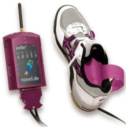
**Figure 6.** Foot-pressure monitoring system, Pedar (Novel, Munich, Germany, [www.novel.de](http://www.novel.de)).
