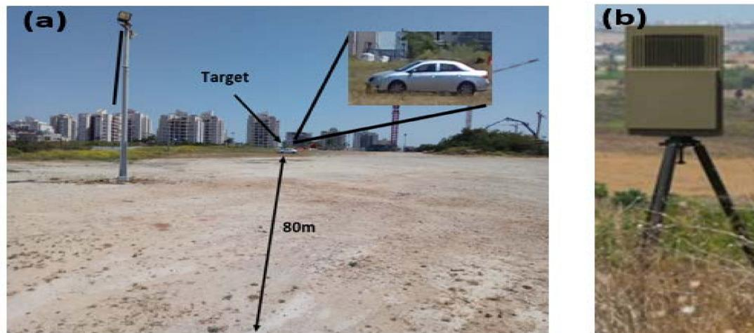
**Figure 1.** (a) View from behind the radar. The target is located 80 m from the radar. The target is shown in the inset; (b) ELTA radar used in the experiment.
